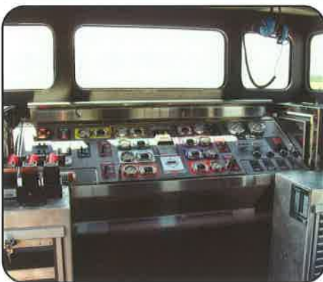
Interior Pump Controls
