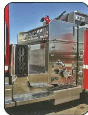
Exterior Top Pump Controls
