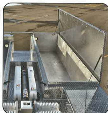
Overhead Storage Bins
